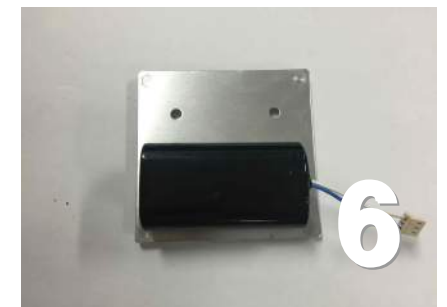
Remove backing on the two way tape from the new battery; center carefully on the two holes and make a little space between two batteries.
