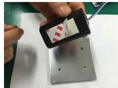
Remove backing on the two way tape from the new battery; center carefully on the two holes and make a little space between two batteries.
