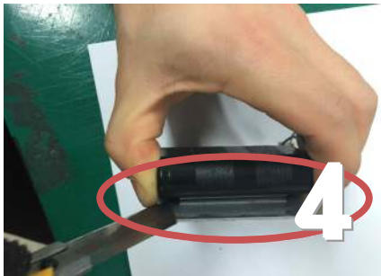
Carefully pry the battery packs off the back plate by using tools such as straight razor
